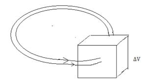
Net out flow of flux per unit volume is zero.
