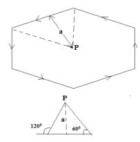
H due to Hexagon is six times the field intensity due to each conductor.
