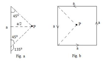
From fig a, the magnetic field intensity due to one conductor is
