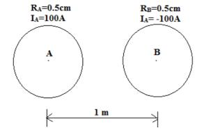
Let  $H_1$  and  $H_2$  be magnetic fields at the surface of conductor 'A' due to the current in conductor 'B'.
