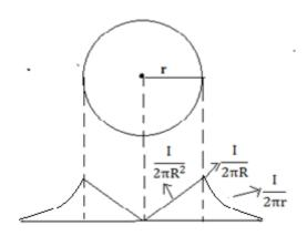
4) A steady current of 100A is flowing in a long straight hollow conductor of inner radius 1 cm and outer radius 2 cm. Assume uniform resistivity. Calculate 'B', the function of radius 'r' from axes of the conductor.
