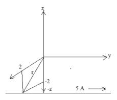
The magnetic field due to a straight current filament  $H=\frac{I}{2\pi r}a_{\emptyset}$
