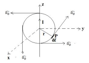
Consider a closed path around a current carrying conductor as shown in fig. The magnetic field at any point on the path is tangent. The point 'P' is at a distance 'r' from the conductor. Consider dl at point 'P' which is at direction  $\widehat{a_{\emptyset}}$  is tangential to the circular path. From the Biot-Savart's law, the M.F.I along the conductor is given by
