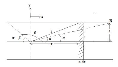
A solenoid has N no of turns on an iron rod. The turns can be assumed to be circular current loops. Considering a small section of length dx at a distance 'x' m from the origin . The no of turns in this section are ndx.
