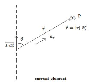
Steady current flowing through a straight conductor produces magnetic field in the form of concentric circles. The magnetic field intensity is given by Biot-Savart's law.
