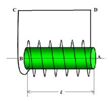
A solenoid has 'N' turns and it carries a current 'I' A. The current direction is shown in fig. The magnetic field is towards left. The magnetic field outside the solenoid is zero.
