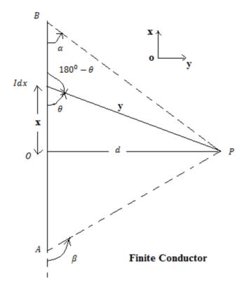
Let dH be the field intensity due to current element Idx which is at a distance 'x' m from the origin.
